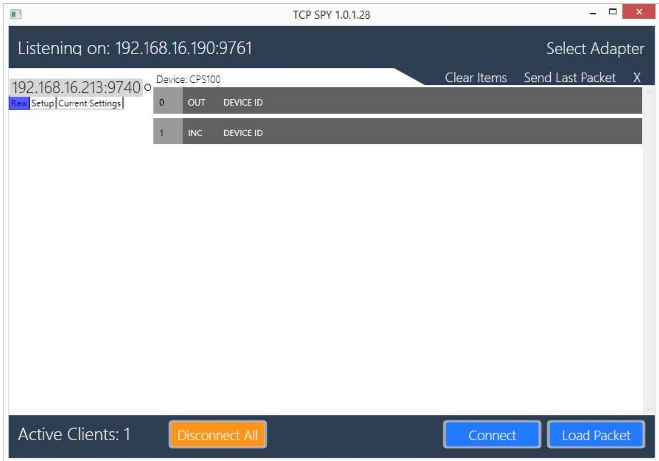
This section shows raw data being sent back and forth. It is used primarily as a CPS100 development tool, and may be safely ignored.
