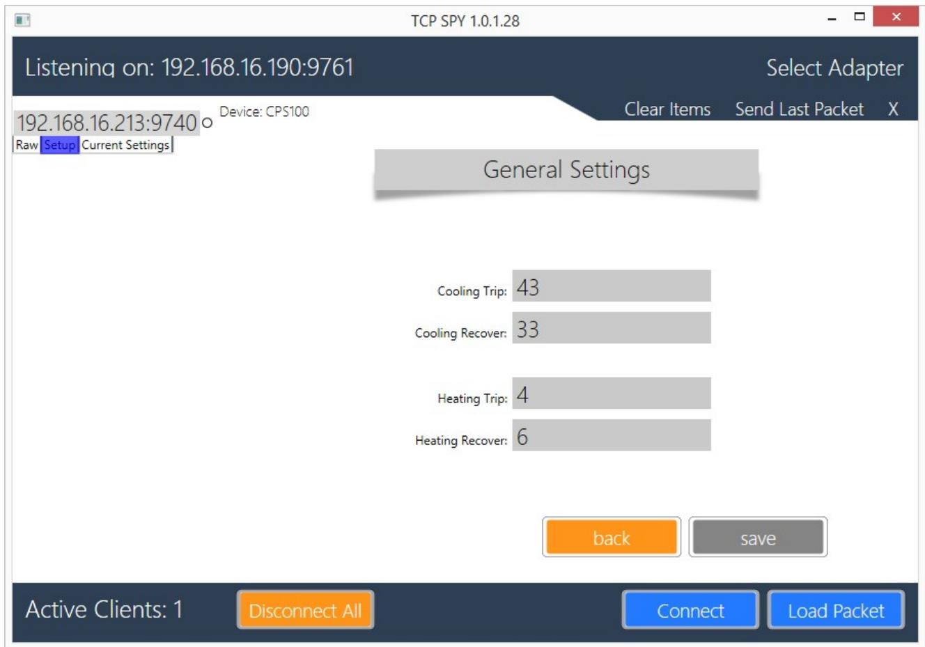
**Cooling Trip:** Sets the point at which cooling fans activate
